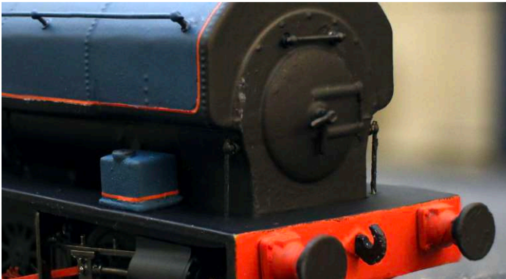
Close-up to show location of smokebox handrail mounting points
