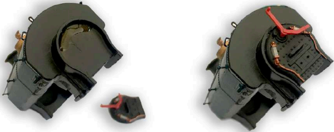
Fitting the firebox backhead to the boiler (demo model shown)
